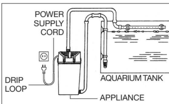
The “drip loop” is that part of the cord below the level of the receptacle, to prevent water travelling along the cord and coming in contact with the receptacle. If the plug or receptacle does get wet, **DON'T** unplug the cord; disconnect the fuse or circuit breaker that supplies power to the appliance. Then unplug and examine for presence of water in the receptacle.
